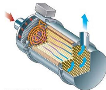
The filter is ready for use when the regeneration process is finished.
